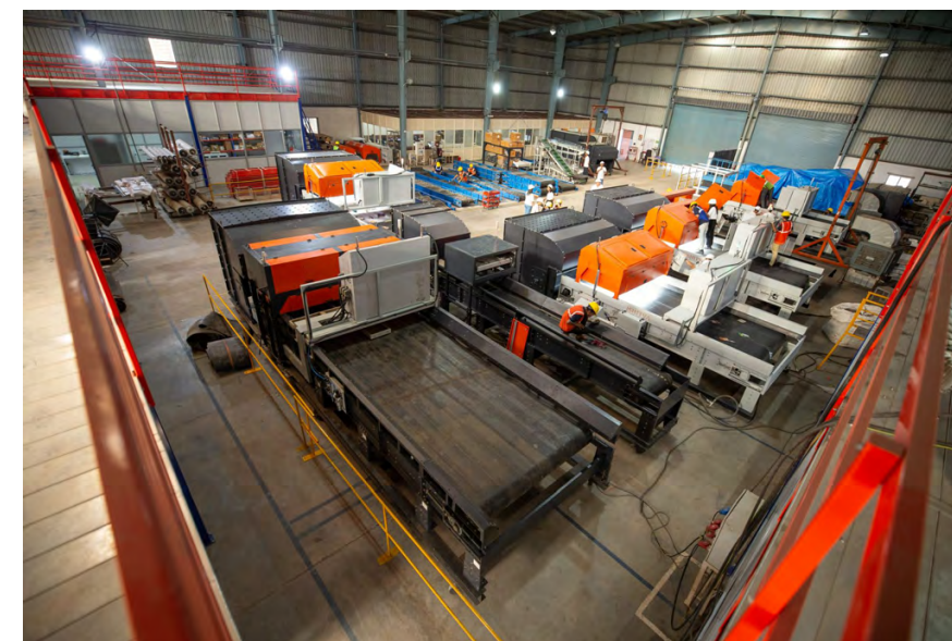
Automated material recovery facility (MRF) using Ishitva's AI-enabled waste sorting line | Image Source: Ishitva
